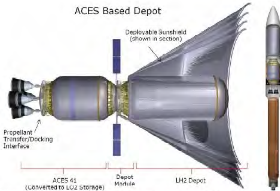
Figure 10. A Single Launch, Dual-Fluid Propellant Depot. Credit ULA
