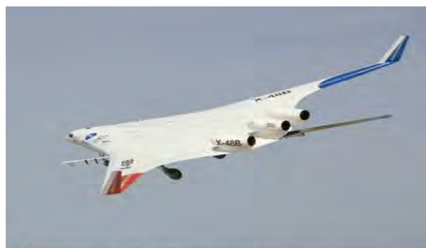
NASA Dryden Flight Research Center Photo Collection http://www.dfrc.nasa.gov/Gallery/Photo/index.html NASA Photo: ED08-0092-03 Date: April 4, 2008 Photo By: Carla Thomas The X-48B Blended Wing Body research aircraft banks smartly in this Block 2 flight phase image.
