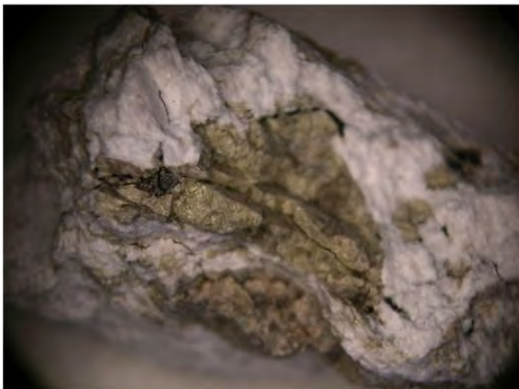
Figure S3. Photograph of initial clast of 60025 analyzed in this investigation. Note the large pyroxene fragment (light green) in the plagioclase matrix (white).
