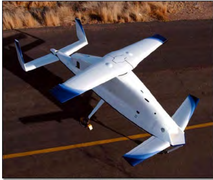
The autonomous Canard Rotor/Wing X-50 Ship No. 1 is currently undergoing testing. First flight of the aircraft is expected later this year.
